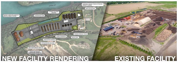
Using a state-of-the-art Aerated Static Pile System and biofilter, the facility composts materials efficiently and effectively with minimal odor. An advanced stormwater reclamation system will allow for water reuse and containment protecting area surface and groundwater.
